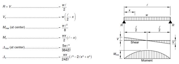
Figure 3 - Design Aid Tables (Beam Design Equations and Diagrams) - PCI Design Handbook
