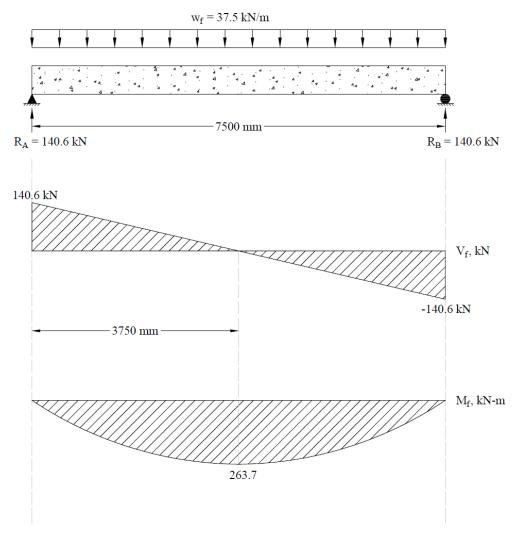
Figure 2 – Shear and Bending Moment Diagrams
